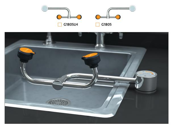
**Application:** AutoFlow<sup>™</sup> eyewash for mounting on counter next to sink. Swinging the spray head assembly 90 degrees horizontally out over the sink activates the water flow. The unit remains in operation until the spray head assembly is swung back into the storage position, closing the valve.
